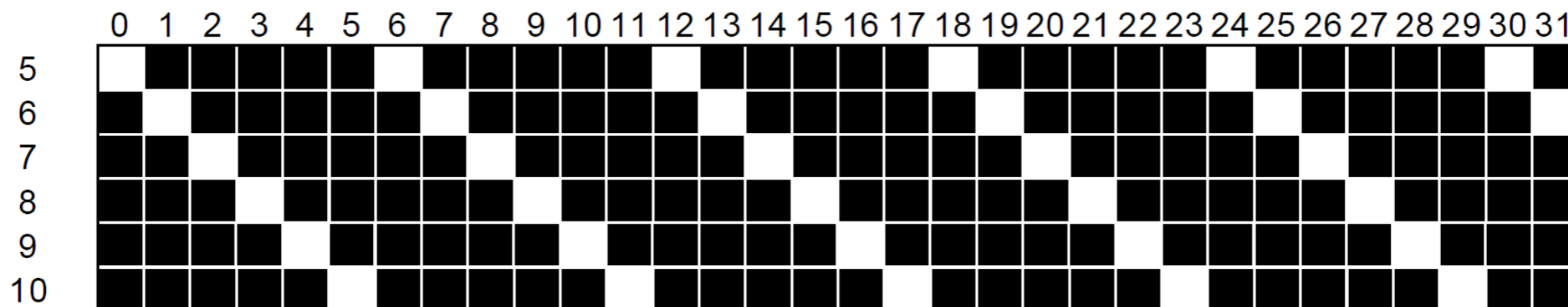
Line Shift Sequence (Pattern Length: 6 Lines)
